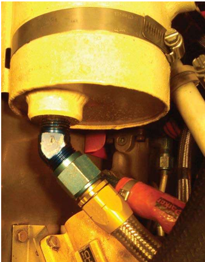
The bottom of the separator and the standard aviation fittings. The blue fitting attached to the separator bottom is an MS20823-10D 1/2-inch male NPT to 5/8-inch (-10) male AN flared aluminum 45-degree fitting. The oil hose is Parker Stratoflex type 156 with a 5/8-inch (-10) female AN flared straight end fitting.
