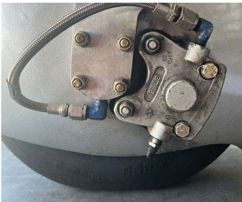
Figure 1. Use wheel bolts slightly longer than stock bolts to allow for the thickness of the metal plate.
