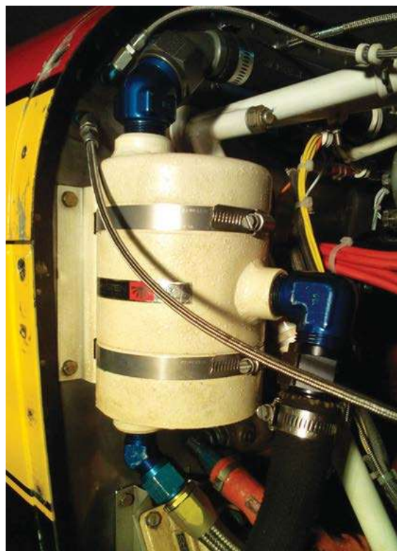
An overall view of my oil separator in place, mounted to the firewall inside of the engine compartment.
