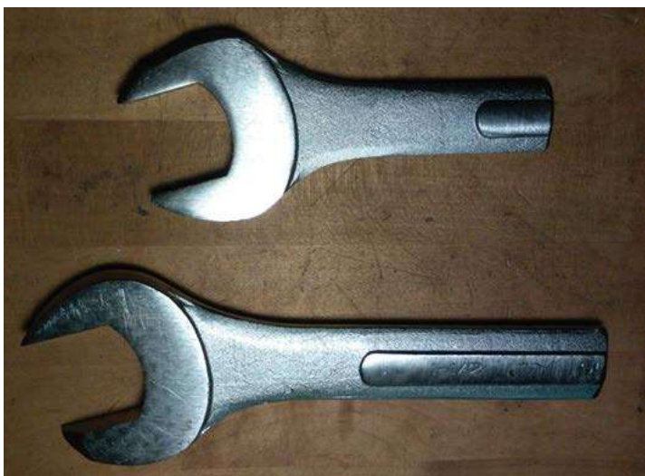
Two inexpensive open-ended wrenches that I purchased and slightly modified (chopped short) with an angle grinder to loosen and tighten the new flared fittings within the available clearances of my engine compartment. I use a second wrench to assure that I do not disturb the sealing of the separator NPT threads.
