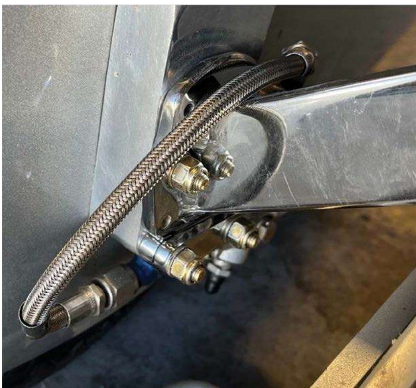
Figure 4. The prototype revealed a minor problem getting the jack plate beneath the hose.
