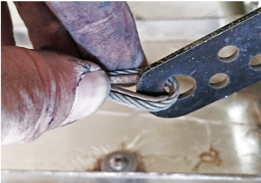
Close-up of the right rudder cable showing complete wear through the thimble and the beginnings of the cable itself being cut through.
