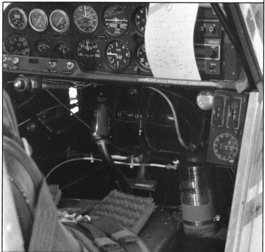
Some lap section of Ken Stout's Hooker Harness is visible in foreground above. Centered under the instrument panel and ahead of the control stick is the header tank with its fuel lines. Below it and mounted on the firewall between the rudder pedals is a Halon bottle for the fire extinguisher system. A round release button is above it to right of tank and just under panel. The photo on page 13 shows Stout in his cockpit wearing his Hooker Custom Harness, parachute, custom fitted helmet and Nomex flight suit and gloves.
